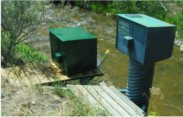
Water quality and flow monitoring station on Clear Creek
